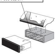
Spacer installation frame 6 mm 7 608 002 076
